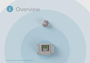
The Wi-Fyre Wireless Optical Heat Detector consists of a ProFyre optical-heat detector head combined with the Wi-Fyre wireless base. The detector uses 'or' logic and is designed to respond to both smoke and/or heat, whichever is triggered first, and is designed and tested in accordance with EN54 parts 5 & 7.
